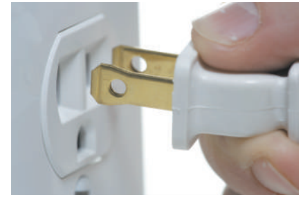
Figure 31.5 This wall socket delivers a root-mean-square (rms) voltage of 120 V.
