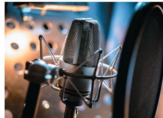
Figure 24.3 Inside a condenser microphone is a capacitor with one rigid plate and one flexible plate. The two plates are kept at a constant potential difference V_{ab} . Sound waves cause the flexible plate to move back and forth, varying the capacitance C and causing charge to flow to and from the capacitor in accordance with the relationship C = Q/V_{ab} . Thus a sound wave is converted to a charge flow that can be amplified and recorded digitally.
