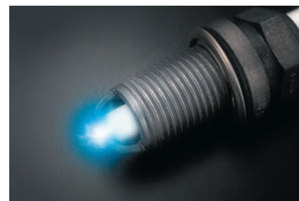
Figure 30.10 The energy required to fire an automobile spark plug is derived from magnetic-field energy stored in the ignition coil.
