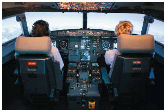
Figure 2.27 The inertial navigation system (INS) on board a long-range airliner keeps track of the airliner’s acceleration. Given the airliner’s initial position and velocity before takeoff, the INS uses the acceleration data to calculate the airliner’s position and velocity throughout the flight.
