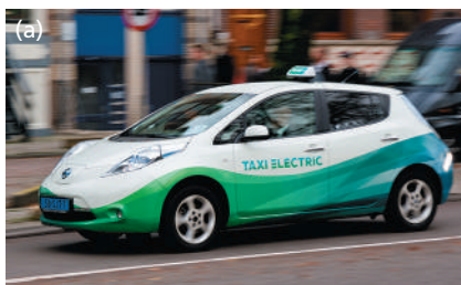
Figure 29.19 Applications of induced electric fields. (a) This car is powered by an electric motor. As the car comes to a halt, the spinning wheels run the motor backward so that it acts as a generator. The resulting induced current is used to recharge the car's batteries. (b) The rotating crankshaft of a piston-engine airplane spins a magnet, inducing an emf in an adjacent coil and generating the spark that ignites fuel in the engine cylinders. This keeps the engine running even if the airplane's other electrical systems fail.
