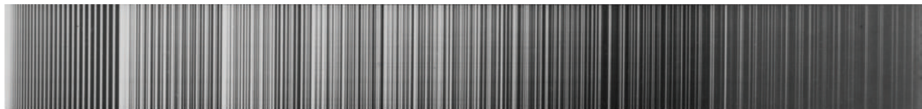
Figure 42.9 A typical molecular band spectrum.
