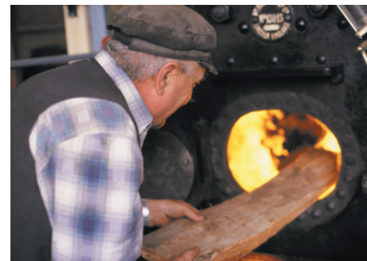
Figure 20.12 The temperature of the firebox of a steam engine is much higher than the temperature of water in the boiler, so heat flows irreversibly from firebox to water. Carnot’s quest to understand the efficiency of steam engines led him to the idea that an ideal engine would involve only reversible processes.
