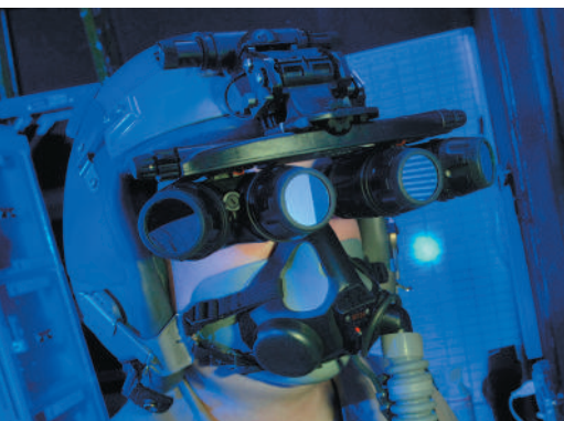
Figure 38.2 (a) A night-vision scope makes use of the photoelectric effect. Photons entering the scope strike a plate, ejecting electrons that pass through a thin disk in which there are millions of tiny channels. The current through each channel is amplified electronically and then directed toward a screen that glows when hit by electrons. (b) The image formed on the screen, which is a combination of these millions of glowing spots, is thousands of times brighter than the naked-eye view.
