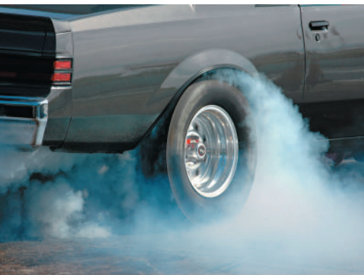
Figure 10.14 The smoke rising from this drag racer’s rear tires shows that the tires are slipping on the road, so v_{\text{cm}} is not equal to R\omega .
