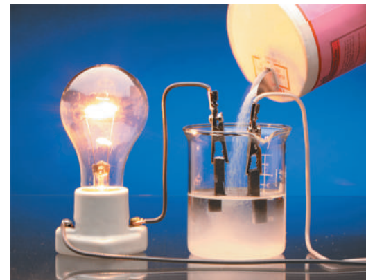
Figure 25.4 Part of the electric circuit that includes this light bulb passes through a beaker with a solution of sodium chloride. The current in the solution is carried by both positive charges ( \text{Na}^+ ions) and negative charges ( \text{Cl}^- ions).
