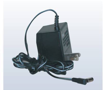
Figure 31.23 An ac adapter like this one converts household ac into low-voltage dc for use in electronic devices. It contains a step-down transformer to change the line voltage to a lower value, typically 3 to 12 V, as well as diodes to convert alternating current to the direct current that small electronic devices require (see Fig. 31.3).
