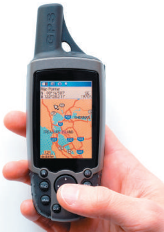
Figure 37.25 A GPS receiver uses radio signals from the orbiting GPS satellites to determine its position. To account for the effects of relativity, the receiver must be tuned to a slightly higher frequency (10.23 MHz) than the frequency emitted by the satellites (10.22999999543 MHz).
