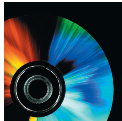
Figure 36.17 Microscopic pits on the surface of this DVD act as a reflection grating, splitting white light into its component colors.
