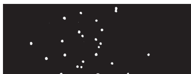
Figure 38.16 These images record the positions where individual photons in a two-slit interference experiment strike the screen. As more photons reach the screen, a recognizable interference pattern appears.
