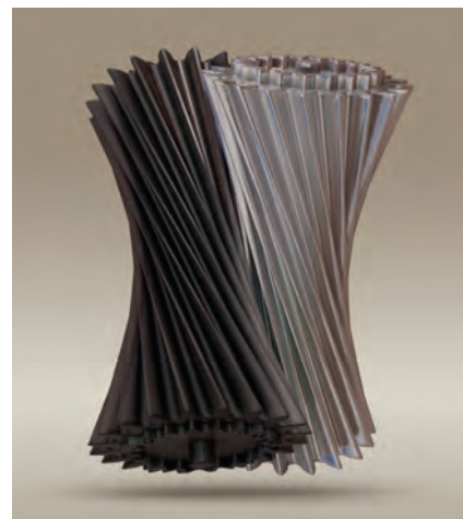
(c) Gears in the shape of hyperboloids mesh and rotate along skew axes.
