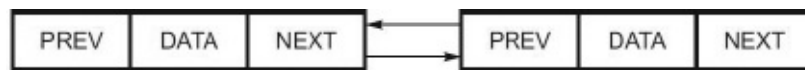
FIGURE 16.8 Node of a doubly linked list are connected via two pointers: NEXT and PREV
