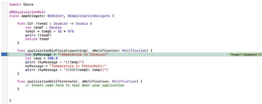
Figure 27-5. A breakpoint halts program execution so you can examine its current state
