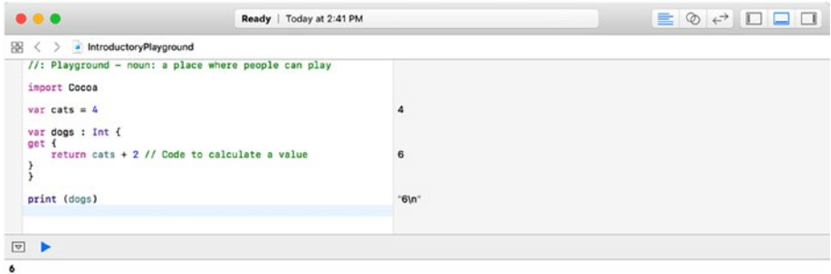
Figure 5-11. The right margin of the playground window shows how the getter portion works
