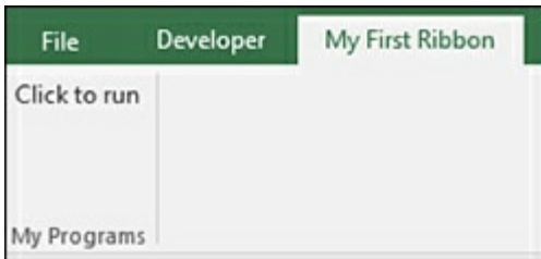
FIGURE 25-2 Run a program with a click of a button on your custom ribbon.
