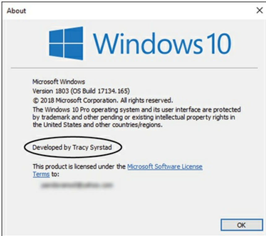
FIGURE 23-2 You can customize the About dialog box used by Windows for your own program.
