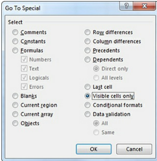
FIGURE 11-3 If rows have been manually hidden, use Visible Cells Only in the Go To Special dialog box.
